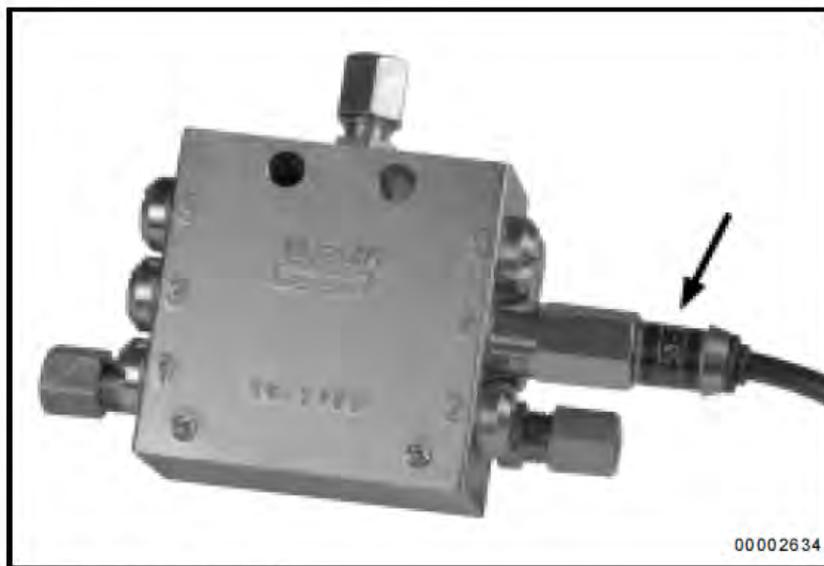
Fig. 20 - Piston detector
