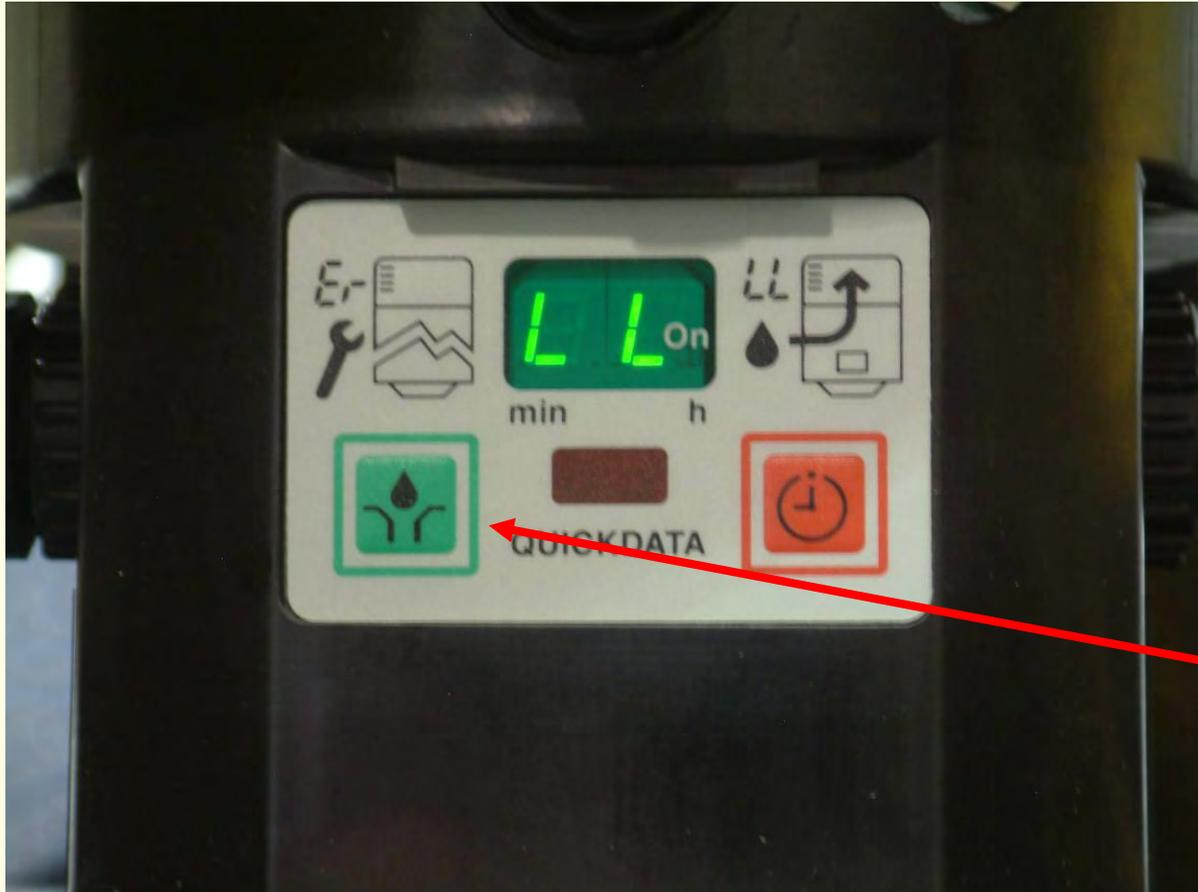
“LL” flashing in display indicates low level in grease reservoir.
