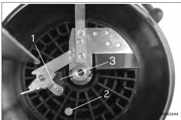
Fig. 33 - Switching parts of the low-level control
