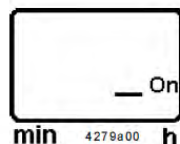
Fig. 23 - Green segment, pause time, voltage applied
