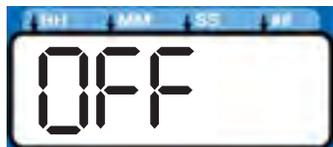
2. Press the UP or DOWN ARROW to change OFF to ON on the display to change the alarm output to be on steady
