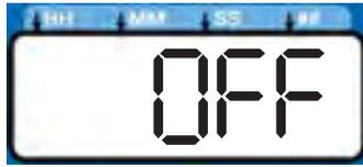
2. Press the UP or DOWN ARROW button to change OFF to ON on the display.
