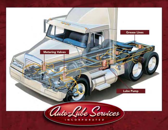
Our expertly installed automated lubrication systems can be adapted to fit on all brands and sizes all sizes and brands of Class 6, 7, and 8 trucks.
