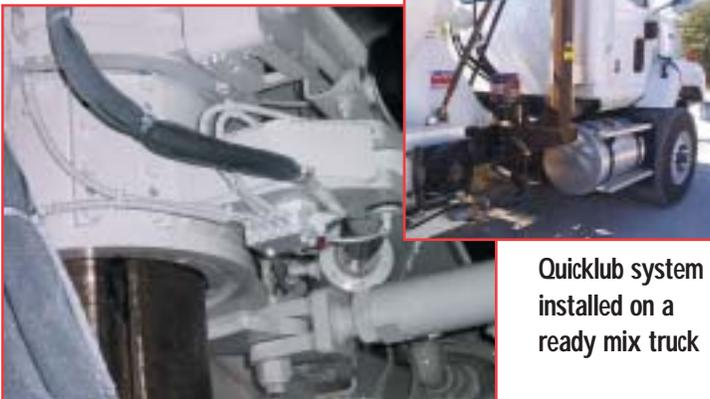
Quicklub system installed on a ready mix truck
