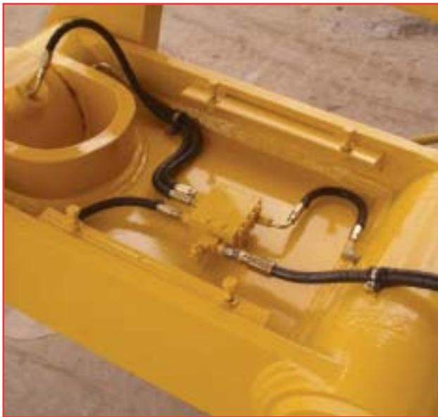
The Quickclub valve is located in the cavity of the H-link. A flat plate of steel will cover and protect the meter valve and hoses
