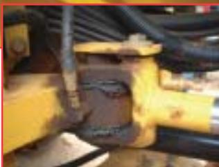
Feedline hoses are protected in “high impact” areas with custom bolt on guarding—note the grease seal that keeps highly abrasive rock and sand out of the bearing
